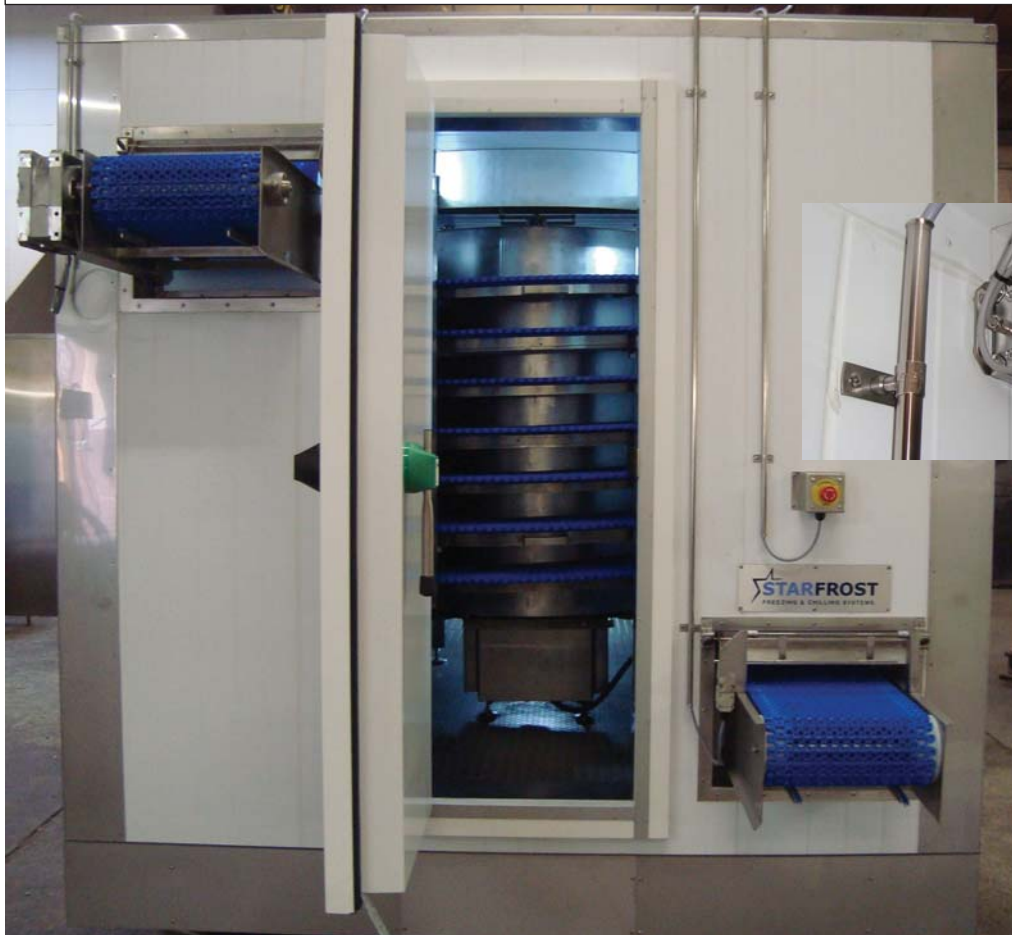
Starfrost's novel spiral freezer unit showing the low-level in-feed and high level exit conveyors, and the spiral freezing zone within
